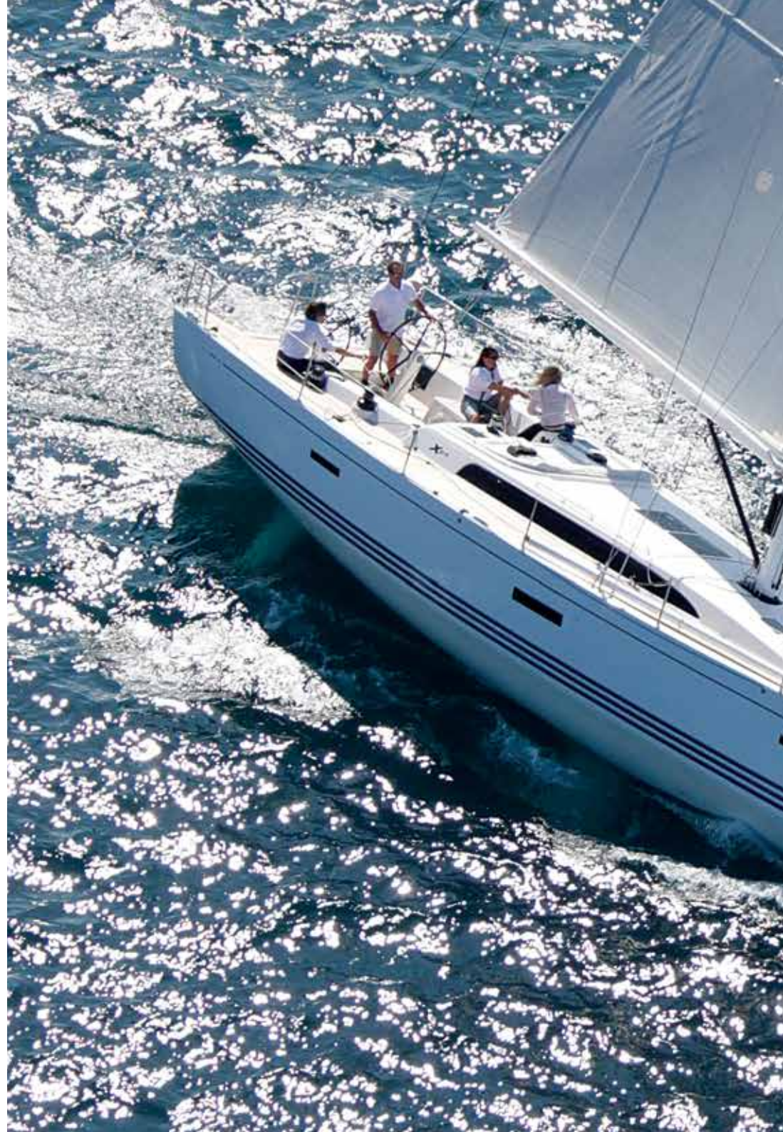
Left and centre: A custom-designed three-spreader alloy rig is supplied as standard, with a higher aspect carbon mast and boom available as an option
