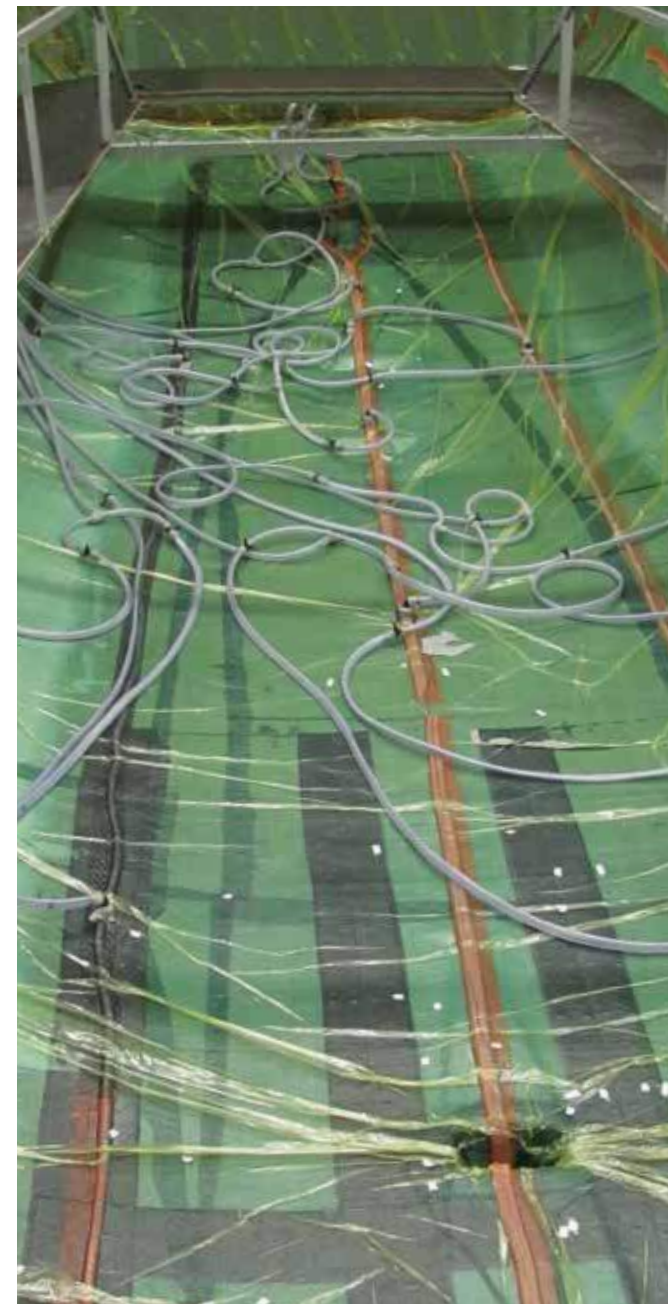
Vacuum infusion build of an Xperformance hull, showing uni-directional carbon tapes in hull laminate
