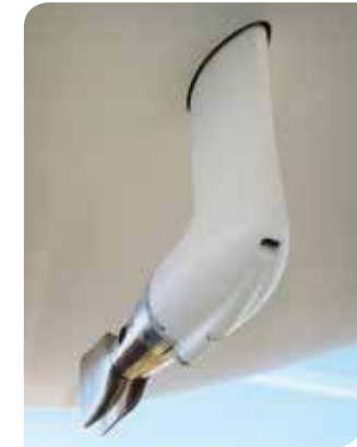
X-Yachts engine struts are faired into the hull for reduced drag and improved reliability
