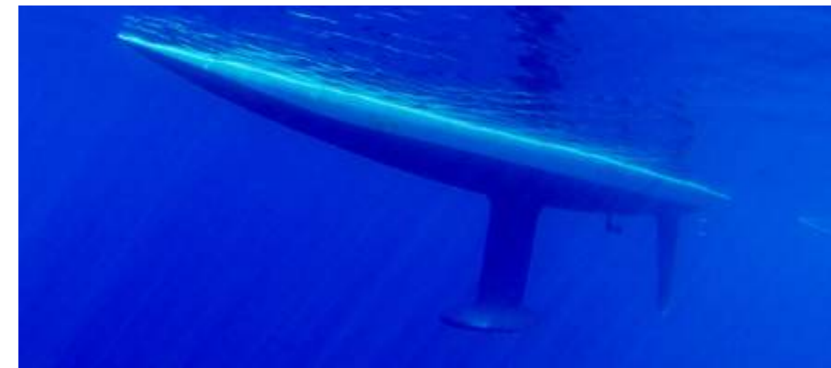
X-Yachts engine struts are faired into the hull for reduced drag and improved reliability
