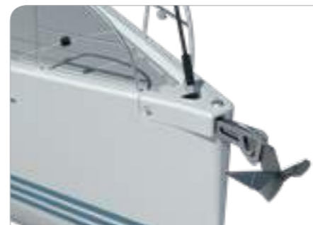
Standard GRP cowl with integrated anchor fitting
