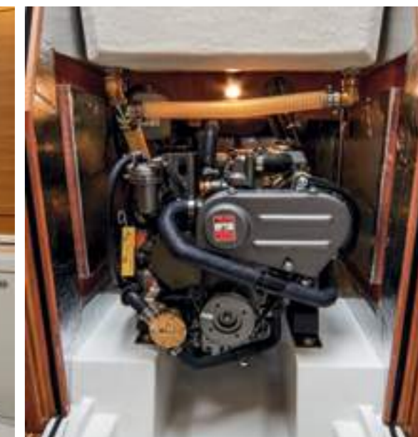
The engine compartment is designed for ease of access and maximum soundproofing
