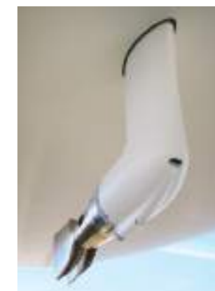
X-Yachts engine struts are faired into the hull for reduced drag and improved reliability
