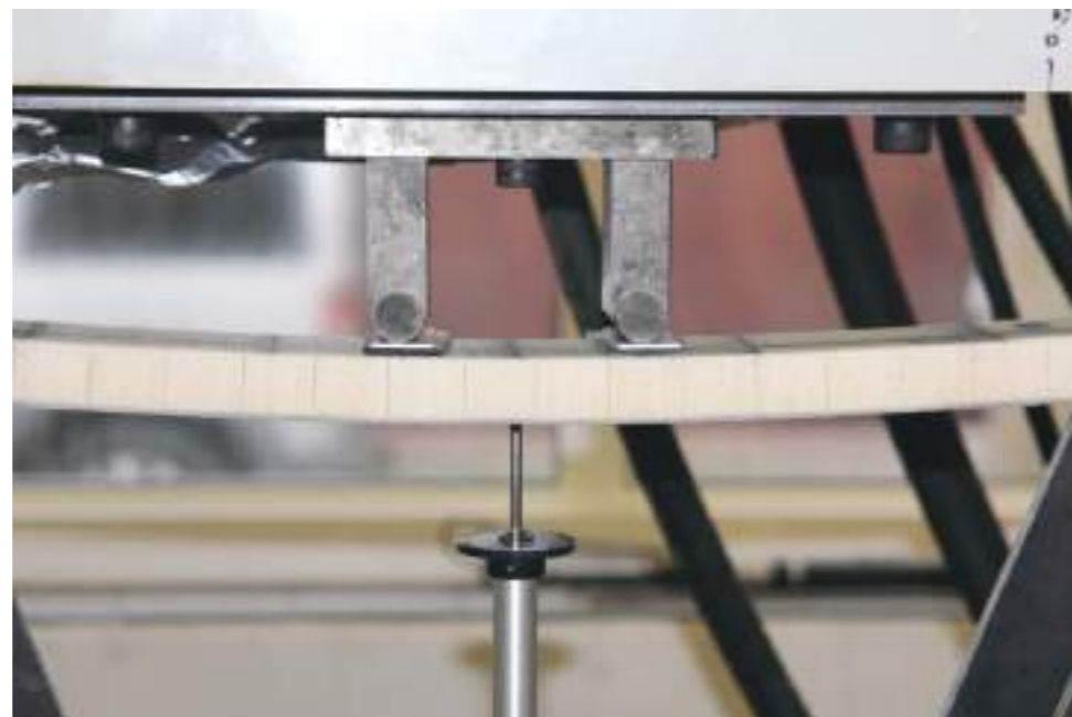
Above: Infused panels undergoing flex testing at the renowned Wolfson Unit MTIA in Southampton – these test panels are just 75mm wide and 600mm long but can withstand a load of 300kgs
