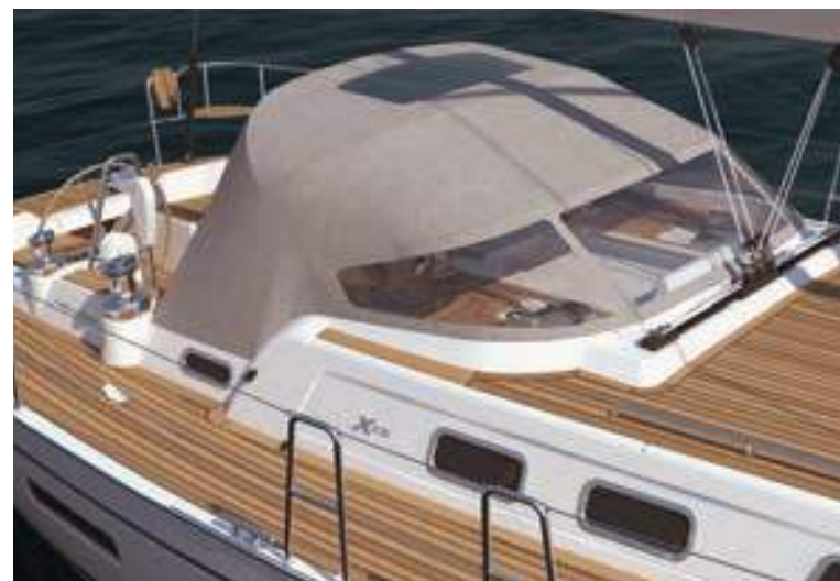
The standard spray hood is supported by three stainless steel frames. For canvas colour options, see pages 22-23.
