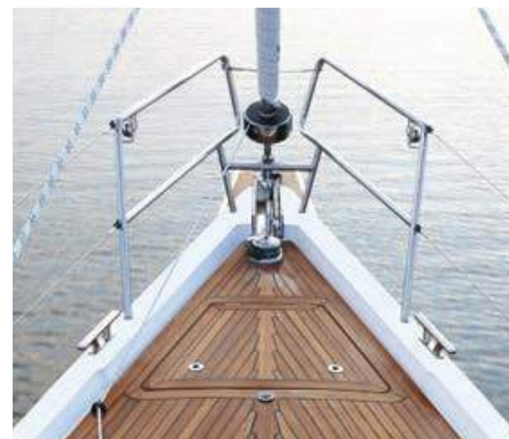
In the foredeck a deep sail locker, with integrated self draining anchor chain compartment. The electric anchor winch capstan can be fitted with an optional topwinch to operate moorings.
