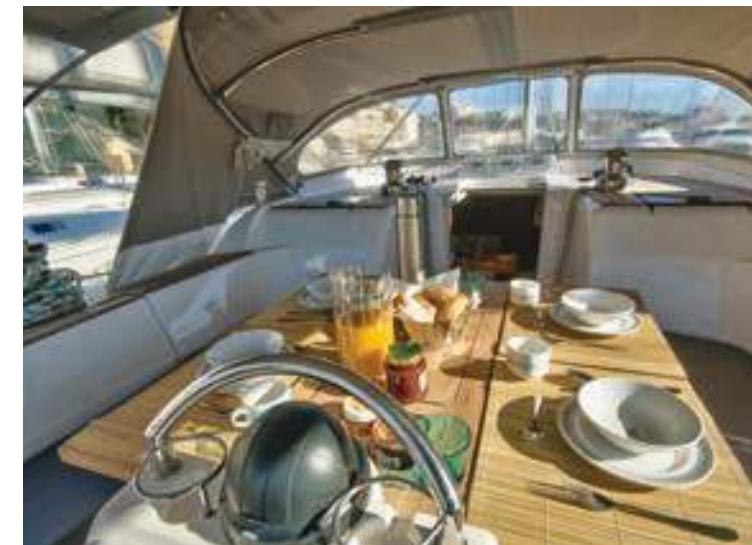
Folding teak cockpit table. Storage in centre of table. Optional grabrail on forward end.
