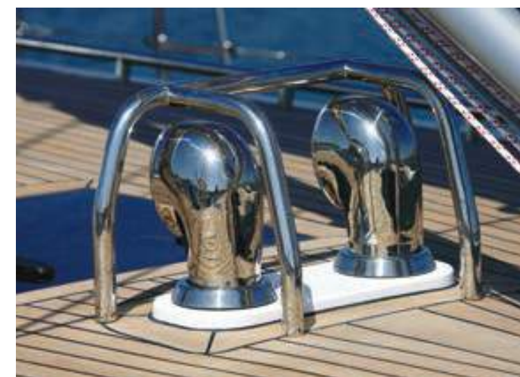
Stainless steel ventilation dorades are mounted on the coach roof, with stainless steel protection bar, provide excellent ventilation into the accommodation.
