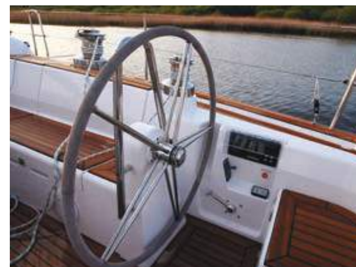
The 'standard' Xc 50 comes with stainless steel wheel crash bars. Optional enlarged crash bars with integrated engine throttle and/or thruster controls on the starboard wheel.
