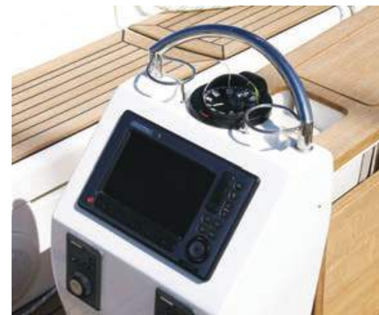
Cockpit table GRP instrument support, designed to fit a chart plotter and binnacle compass.
