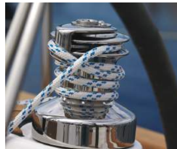
Stainless steel self-tailing Andersen Winches, which can be upgraded to be electrical powered are part of Xc 38's comprehensive standard quality.
