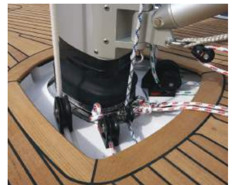
Optional vacuum applied teak (alternatively Flexiteak, see price list for details) on the coachroof. Split mainsheet passes below deck on both sides and is led back to the aftmost cockpit winches.
