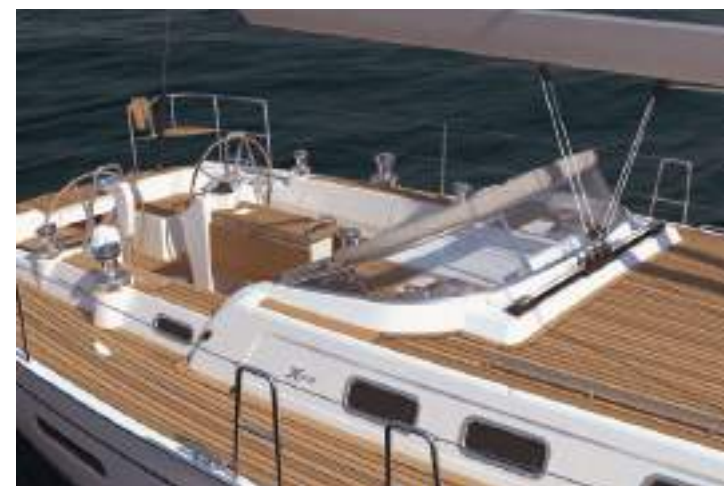
The Xc 38 comes with an optional aluminium framed windshield made from toughened glass including a stainless steel framed sprayhood.
