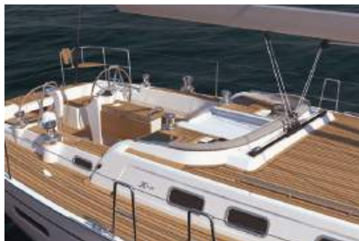
The spray hood resting in a "sock" when folded. The aft pushpit teak seats are standard.
