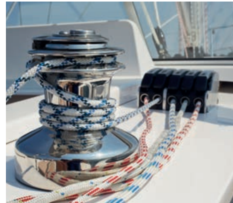
The Xc 35 comes standard with 6 self-tailing Harken winches. Optional stainless steel Andersen winches are available as an upgrade.
