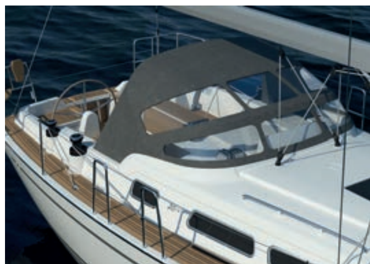
The spray hood is supported by three stainless steel frames. For canvas colour options, see page 17.
