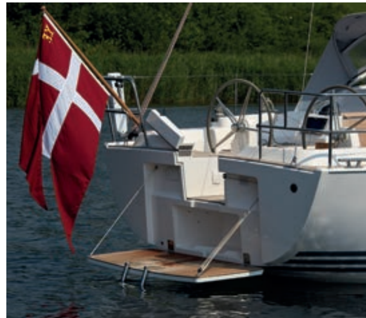
The large bathing platform is operated by a purchase block system. Below deck storage for a liferaft is accessed from the bathing platform.
