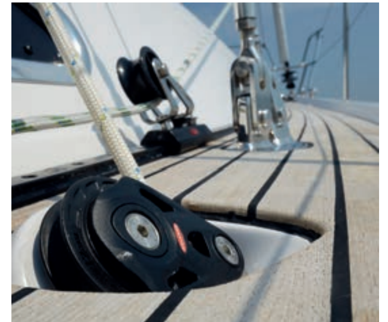
A vacuum applied teak side deck can be added. German mainsheet passes below deck on both sides and is led back to the aftmost cockpit winches.
