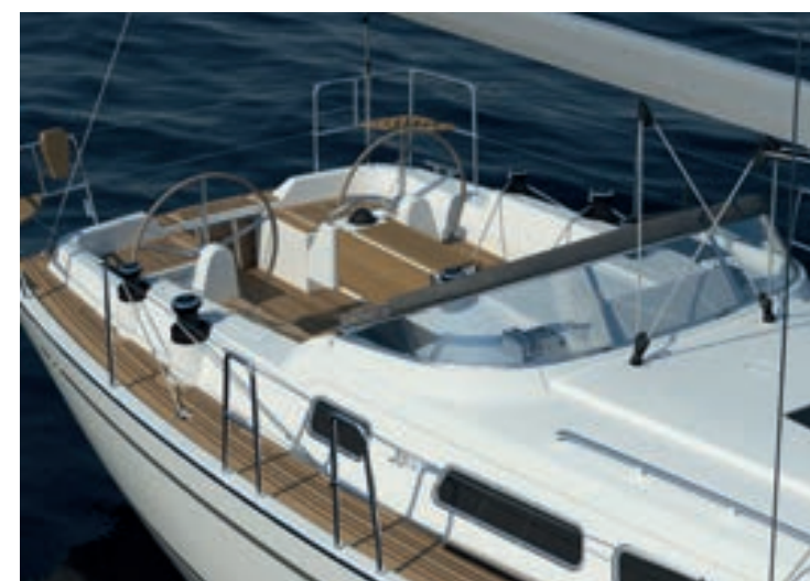
Xc 35 comes with an aluminium framed windshield made from toughened glass including a stainless steel framed sprayhood.
