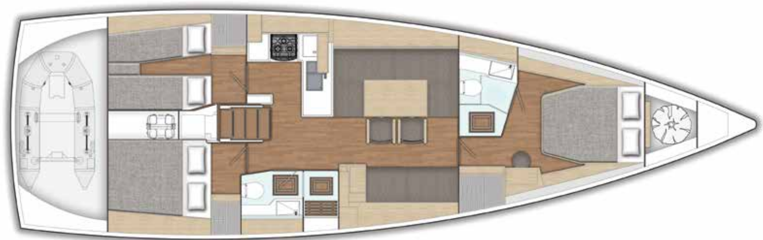
Optional Layout - double & twin cabins aft, aft facing chart-table with dedicated shower compartment in the aft heads
